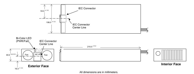
Figure 2: Alternate Enclosure Drawing
